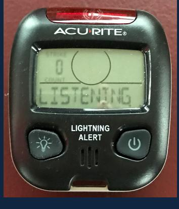
The AcuRite Model 02020 (\$29) is a handheld lightning detector with a monochromatic display of strike count, both cloud-tocloud and cloud-to-ground lightning detection, and an 8-10 month battery life.
