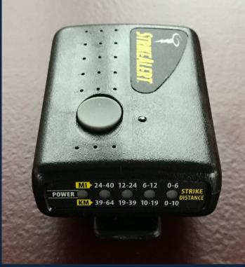
The StrikeAlert LD1000 (\$90) is a handheld lightning detector with LED light detection display, up to 100 hours of battery life, and can only detect lightning in the upright direction.
