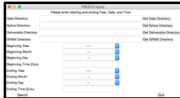
Figure 9. PRESTO data input GUI where the user selects the desired date range and directories to search for atmospheric profiles.
