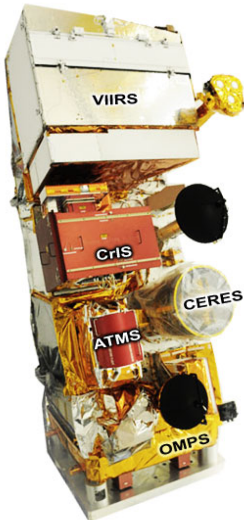
Figure 1. Photo image of the NASA Suomi-NPP satellite with labels for the five sensors. ( https://jointmission.gsfc.nasa.gov/cris.html )
