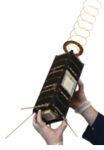
Figure 1: GOMX-3 in fully deployed configuration with helical ADS-B antenna.
