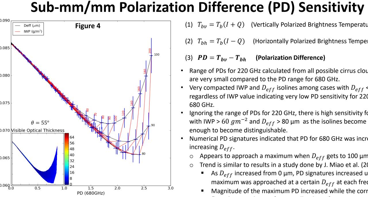
Figure 4: IWP (red) and  $D_{\rho ff}$  (black) isoline plot of PDs with respect to 680 GHz and 220 GHz. The potential error lines (blue) are centered at all intercepts of the IWP and  $D_{eff}$  isolines. The visible optical thickness ( $\tau$ ) contour subplot contains axes of the same scale as the main plot. The viewing zenith angle ( $\theta$ ) is 55°.
