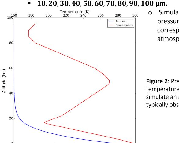
600 Pressure (hPa) • Simulated atmosphere composed of pressure and temperature corresponding to a typical tropical atmosphere (Figure 2).
