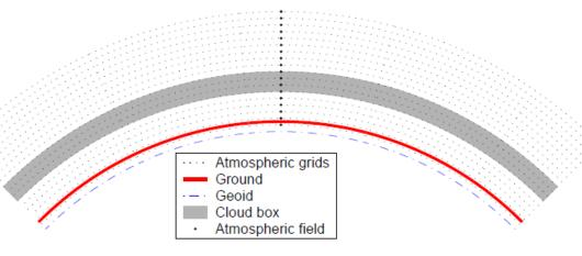
Figure 1: Schematic of a 1D atmosphere implemented in ARTS with a cloud box. The radius of the ellipsoid, the surface and all pressure levels are constant around the globe (Buehler et al. 2017).
