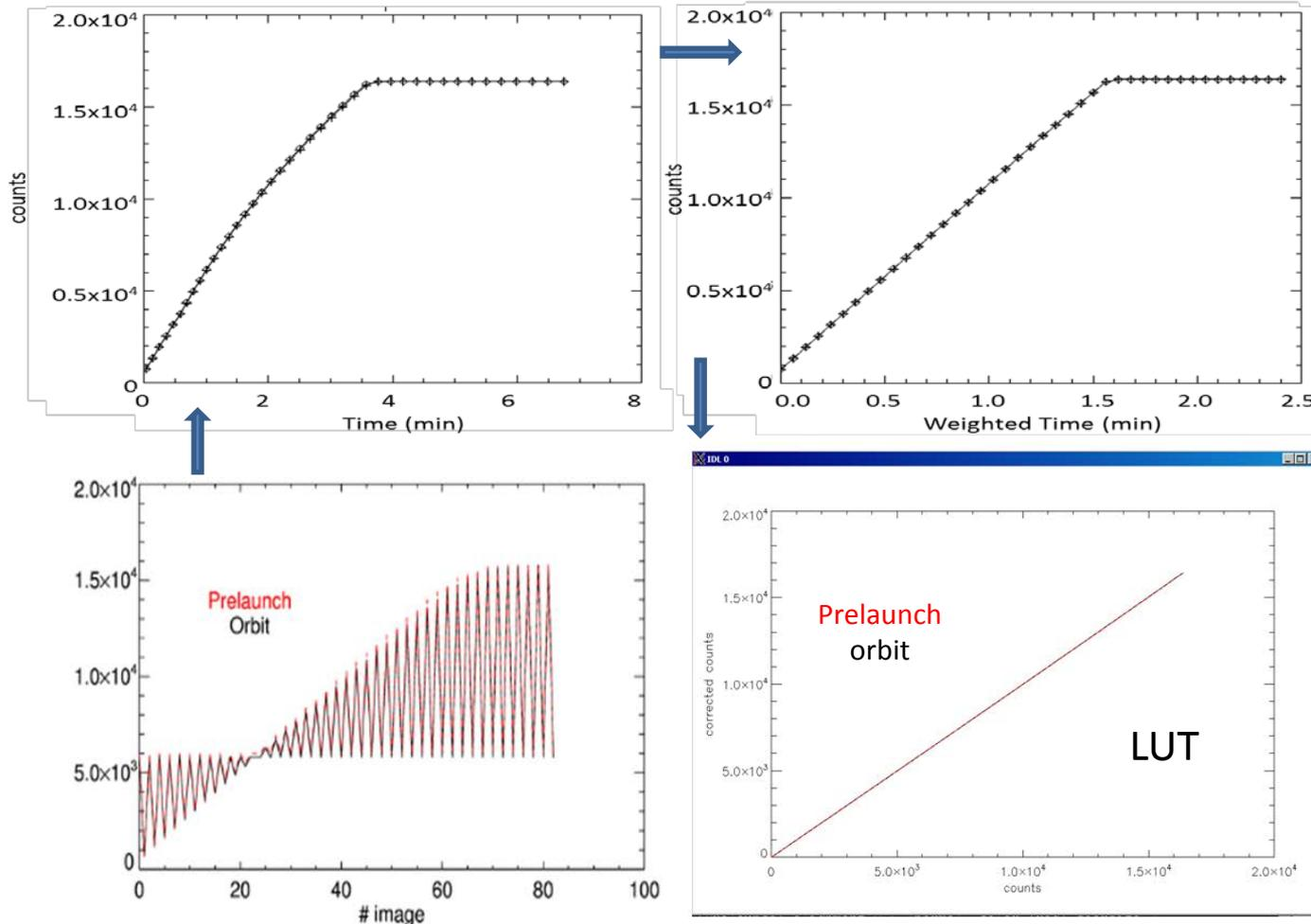
NOAA-20 OMPS system linearity is nearly identical before and after launch
