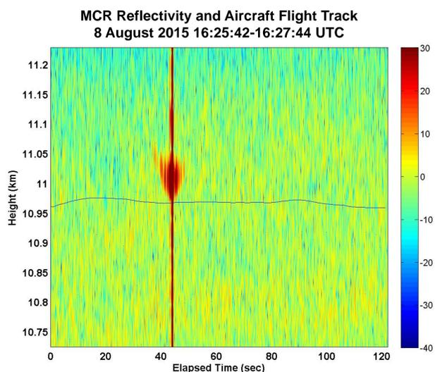
A volume scan from the MCR showing reflectivity (shading, values in dBZ) and the track of UND's Cessna Citation II Research Aircraft (blue line) on a time-height plot. The maximum in the MCR reflectivity is the aircraft as it passes over the MCR. Differences in height between the MCR and aircraft is due to an issue with the range gate spacing on the MCR.
