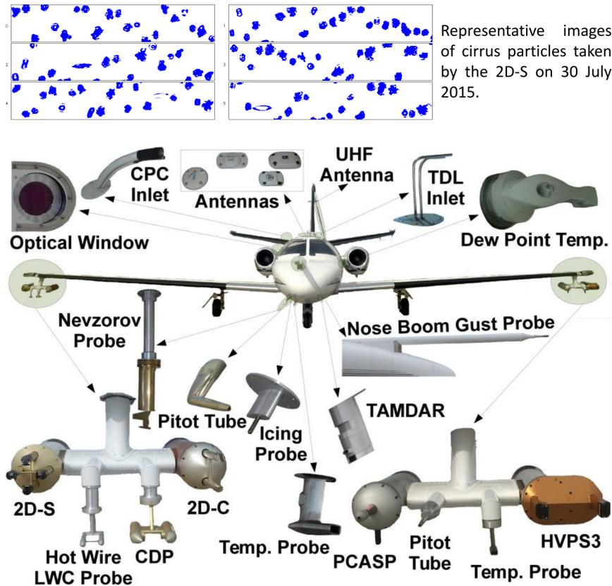
Locations of external instruments onboard the Citation Research Aircraft are shown above. The 2D-S probe provides two-dimensional images of particles using 128 10-um diode lasers with one laser oriented horizontally and one oriented vertically. The Nevzorov Probe measures total and liquid water using hot wire sensors and provides highly accurate total particle mass after processing using routines from the Airborne Data Processing and Analysis software package (Delene, 2011).
