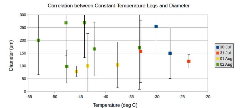
Plot showing average liquid-equivalent diameter from the same flight legs and criterion as above.
