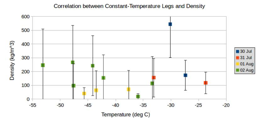
Plot showing the average bulk ice density from 14 flight legs during four CAPE2015 research flights where the temperature remained constant below -20 °C. Error bars show high variability in the density data. Since no correlation is found between temperature and density, the average value is used for synthesizing Nevzorov mass for calculation of reflectivity data for the 8 August 2015 case day.
