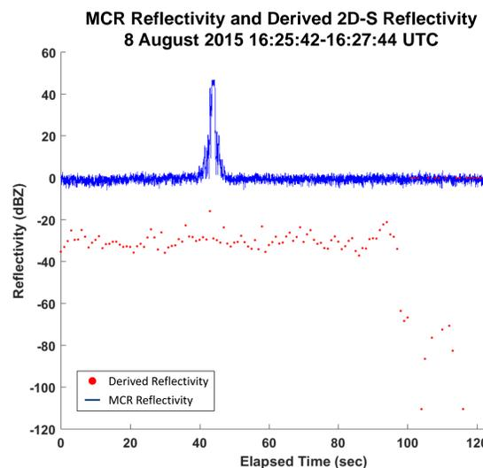
A case where the comparison between the derived aircraft reflectivity and the measured MCR reflectivity shows a difference of 30 dBZ. The MCR reflectivity is averaged over a 500 m column surrounding the aircraft's mean altitude. The spike in MCR reflectivity (about 45 s) is due to contamination of the signal by the aircraft. Generally, the measured MCR reflectivity ranges from -20 to 40 dBZ and aircraft derived reflectivity ranges from -50 to 10 dBZ.
