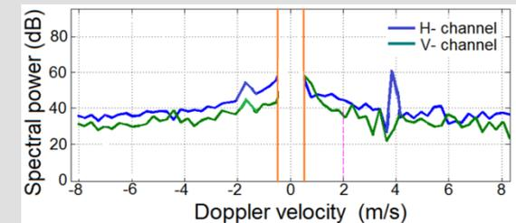
Standard processing: suppress ground clutter
