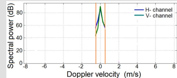
Calibration monitoring: Leave 3 central spectral lines
