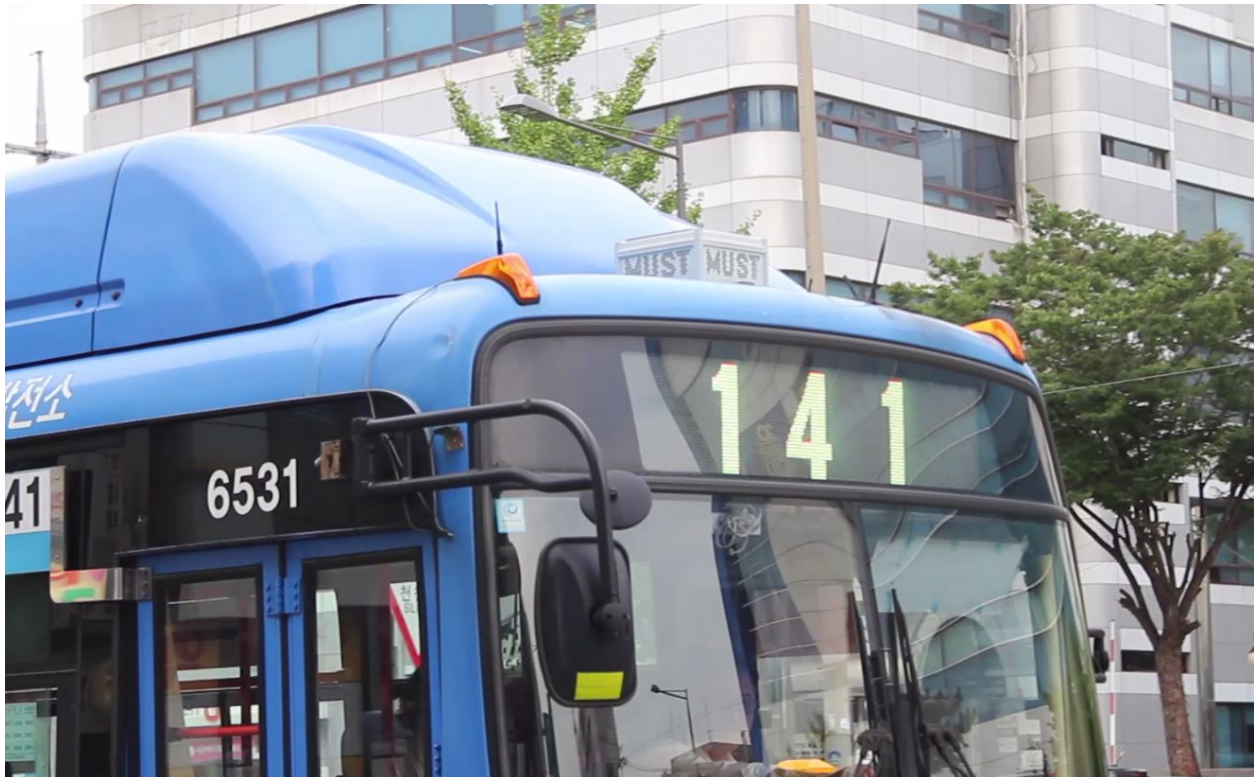
Mobile Urban Sensing Technologies (MUST) sensing kit mounted over Seoul City bus network
