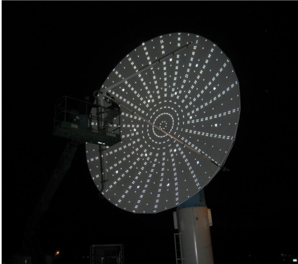
Figure 5: *S-pol antenna surface measurements .*
