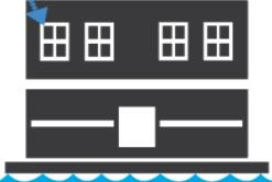
The ground floor is raised 30 inches above the current 500-year flood level and 42 inches above the 100-year flood level.
