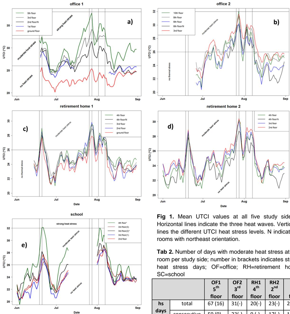
**Fig 1.** Mean UTCI values at all five study sides. Horizontal lines indicate the three heat waves. Vertical lines the different UTCI heat stress levels. N indicates rooms with northeast orientation.
