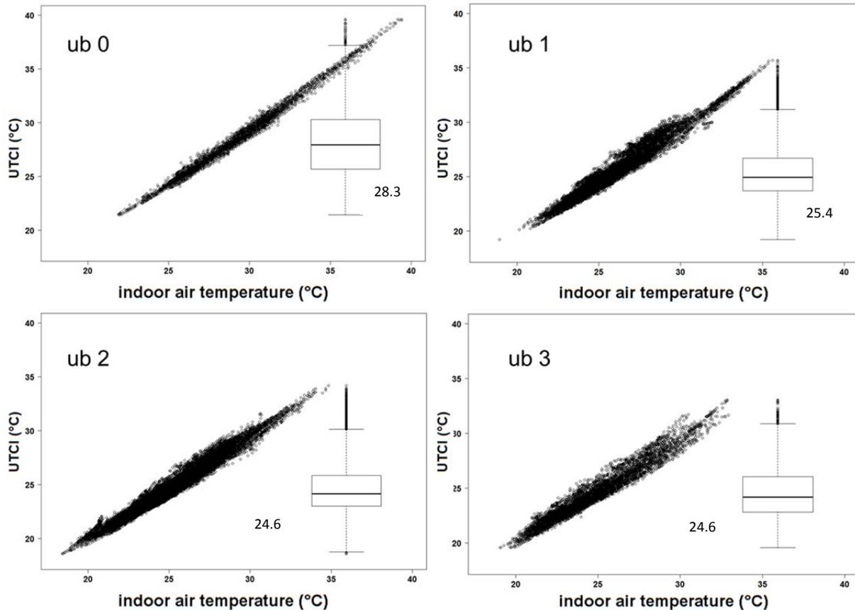
**Fig 3.** The influence of different user behavior patterns on the UTCI and indoor air temperature; the variance of UTCI is additionally expressed by a boxplot diagram; the number indicates the mean UTCI in °C
