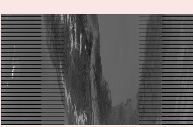
SDR (Sensor Data Record) granules are generally 6-minute segments of data. The images above provide a sample of how large that is (left) and the raw image of the data swaths (with trimmed portions of swath in black). Data for each channel are stored separately as is the geolocation information.
