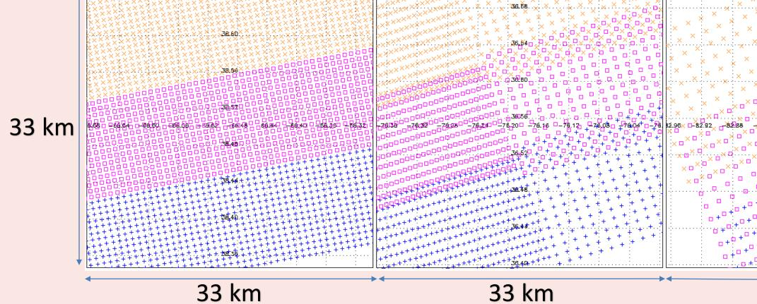
The push-broom design of each swath results in scanlines diverging at swatch edge (the "bow" tie" effect). This results in pixels between swaths overlapping to a large degree, even after satellite providers trim certain portions of lines. This spatial pattern diverges from AVHRR-like simpler data.
