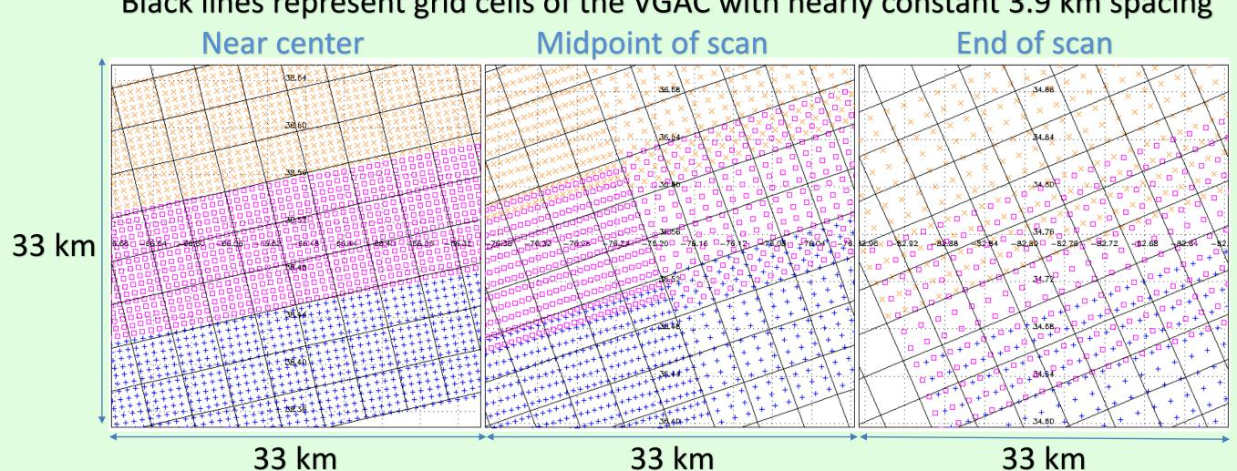
An equal area grid is defined parallel and perpendicular to the satellite track. Grid size remains constant for the entire scan length. Provide same geolocation data as current SDR (lat, lon, solar and viewing angles). For IR and VIS channel, will also store sub-grid cell variability. Can map a position to satellite grid cell using equations (allows forward and backward mapping).
