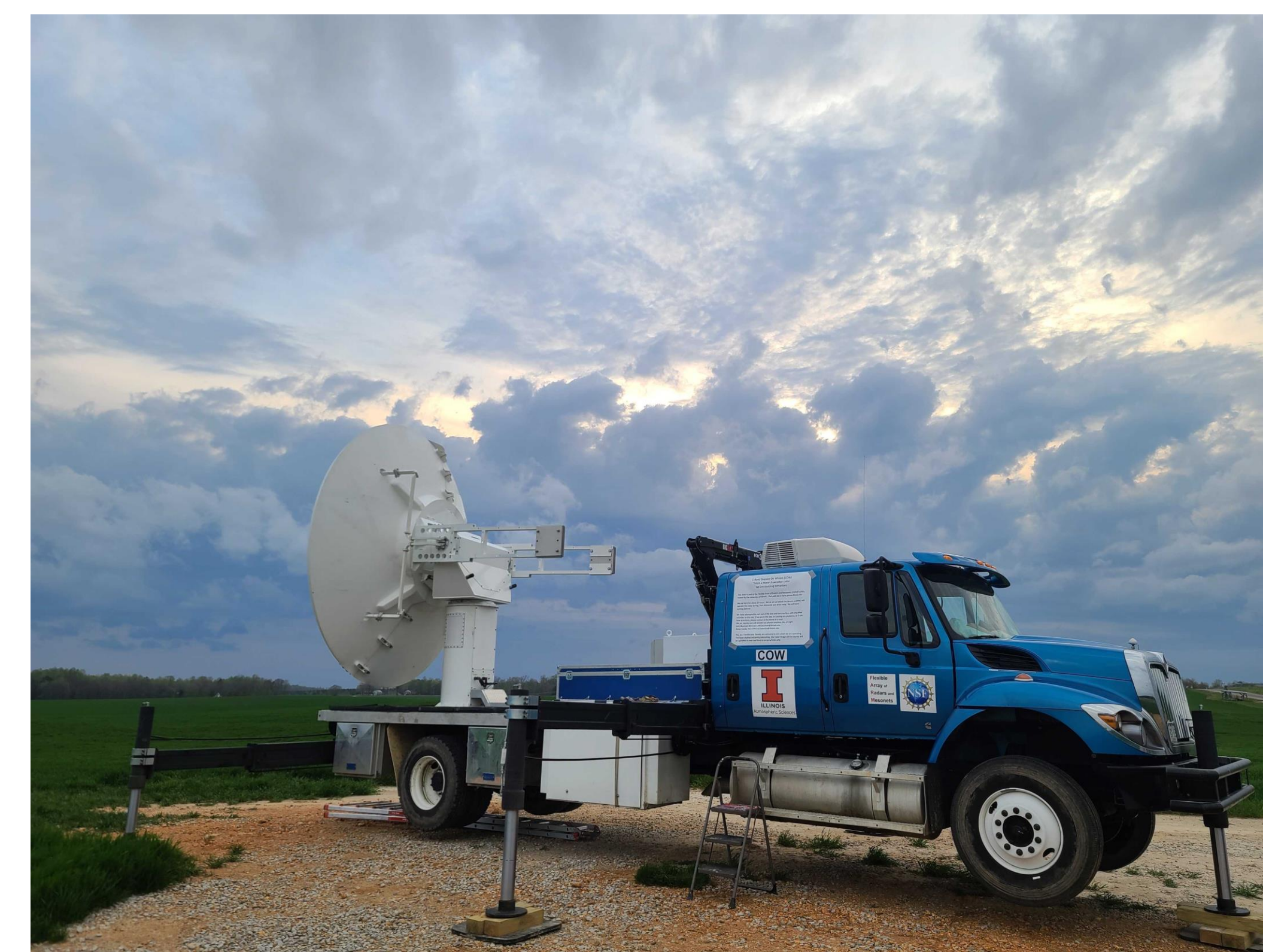
FIG. 3. UIUC FARM's mobile C-band radar (COW1). Photo by Josh Aikens
