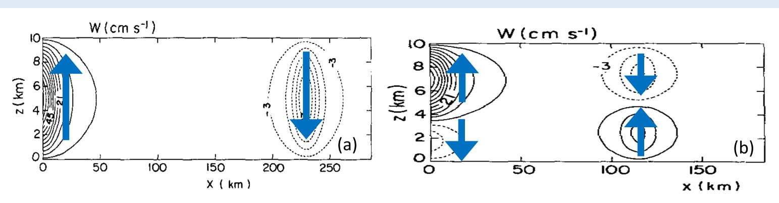
Vertical velocities induced by a (a) 2 J kg<sup>-1</sup> s<sup>-1</sup> convective heating source and (b) 1 J kg<sup>-1</sup> s<sup>-1</sup> stratiform dipole heating source at x = 1. Figure made 2 hours after initiation. Contours are 3 cm s<sup>-1</sup>. Adapted from Nicholls et al. (1991)
