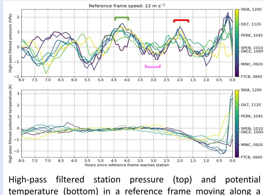
temperature (bottom) in a reference frame moving along a vector from station FTCB to FORA at 22 m s-1. The times (UTC) when the start of the reference frame reaches each station (hour 0) is identified in the color bar. Time increases to the left.
