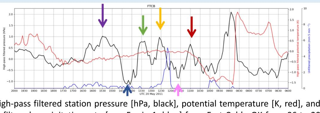
High-pass filtered station pressure [hPa, black], potential temperature [K, red], and unfiltered precipitation rate [mm 5 min-1, blue] from Fort Cobb, OK from 06 to 20 UTC on 20 May 2011. The arrows indicate potential gravity wave perturbations. Time increases to the left
