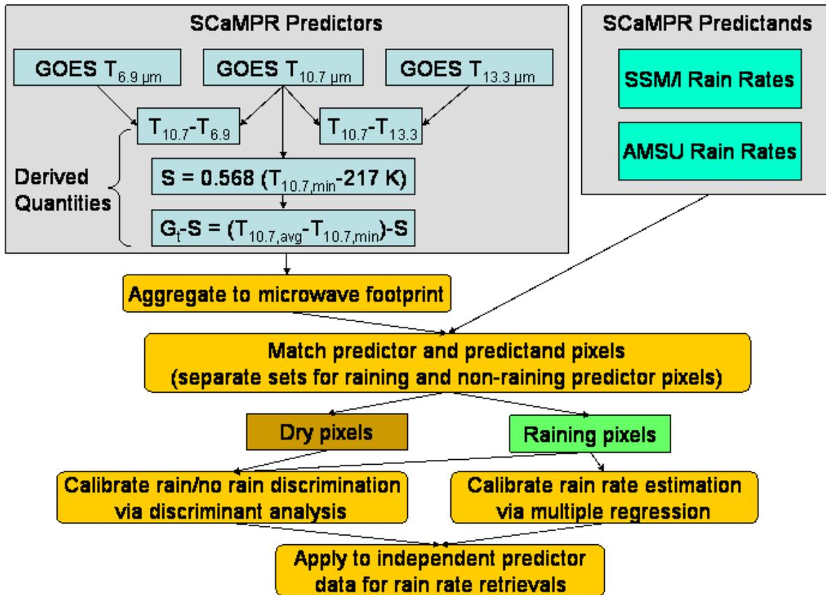
**Figure 1.** Schematic diagram of the SCaMPR algorithm.
