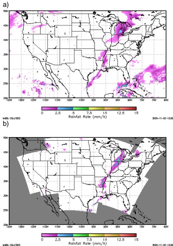
**Figure 2.** Sample SCaMPR 1-h total rainfall field (a) and corresponding Stage IV radar/rain gauge field (b) for 0800-0900 UTC 1 November 2005.
