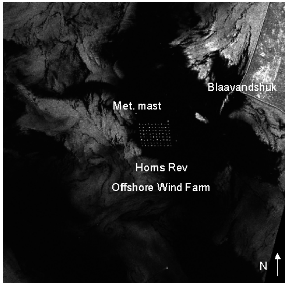
Figure 2. ERS-2 sub-image (50 km x 50 km) showing Horns Rev Offshore Wind Farm in the North Sea, Denmark under calm conditions. Bright areas offshore are not associated with the wind (Christiansen and Hasager 2005).
