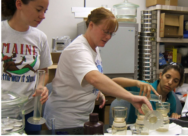
Figure 5: Laboratory work included measurement of total suspended solids in water - which affects water clarity. The resuspension of bottom sediments by the wind has an important effect on sea-grass health in the Indian River Lagoon.
