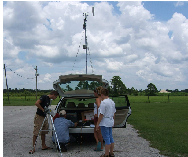
Figure 3: Sea breeze study field data collection included measurements of surface wind speed and direction, downwelling solar radiation, and cloud base temperatures from an infrared thermometer in the vicinity of the sea breeze front.
