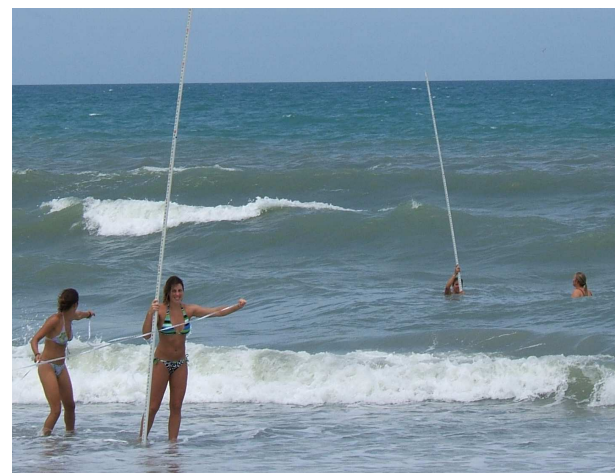
Figure 4: Using differential leveling surveys and determining sand grain-size distribution (not shown), the changing nature of beaches from the dune crest into the surf zone is documented.
