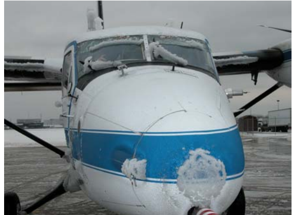
Figure 5: The NASA Glenn Twin Otter Research Aircraft after a successful icing mission.
