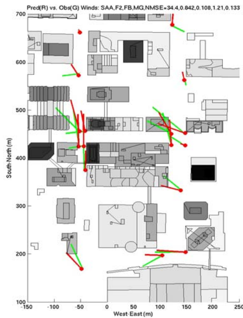
Fig. 6. Comparison of predicted wind vectors (red arrows) against 30-min average data (green arrows) measured by DPG PWIDS on z=8 m plane for IOP 8.
