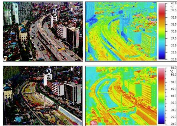
Fig. 1 The change of thermal environment by Cheonggye stream restoration. Right-hand pictures are taken by Thermography. The upper part of figures denotes before restoration (2003) and lower part of figures denotes after restoration (2005).
