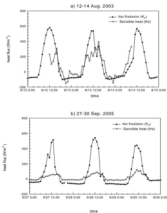
Fig. 4 Comparison of energy fluxes (net radiation ( $R_N$ ) and sensible heat flux ( $H_s$ )) for the before (2003) and after (2005) restoration of Cheonggye stream.
