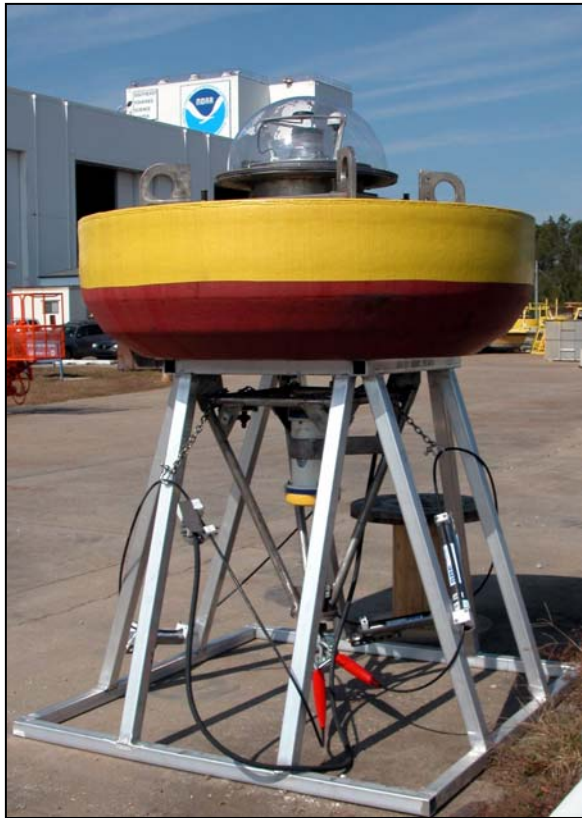
FIG 1. NDBC 1.8m foam buoy (on stand). Contains angular rate sensor, onboard processor, and Iridium communications for directional wave measurement. Can also be outfitted with acoustic current profiler and CT sensor “string.”
