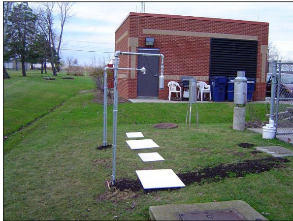
Figure 3. Site configuration of the Judd and Campbell sensors and manual observations in Buffalo, NY.
