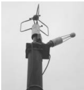
Photo 2: Turbulent measurement sensors on the top of the tower.
