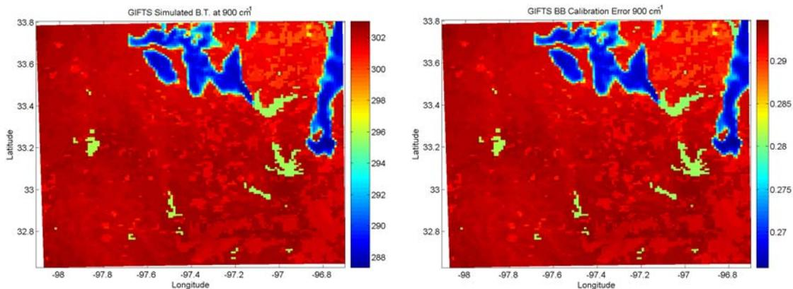
Figure 9. A brightness temperature image of a simulated GIFTS Earth scene (left panel) is shown for the center of the longwave band (900 cm<sup>-1</sup>). The internal blackbody calibration error at 900 cm<sup>-1</sup> is shown in the right hand panel as an image using the uncertainties given in Table 1. The variation in window scene temperature is caused by presence of clouds in the simulation. All units are in Kelvin.
