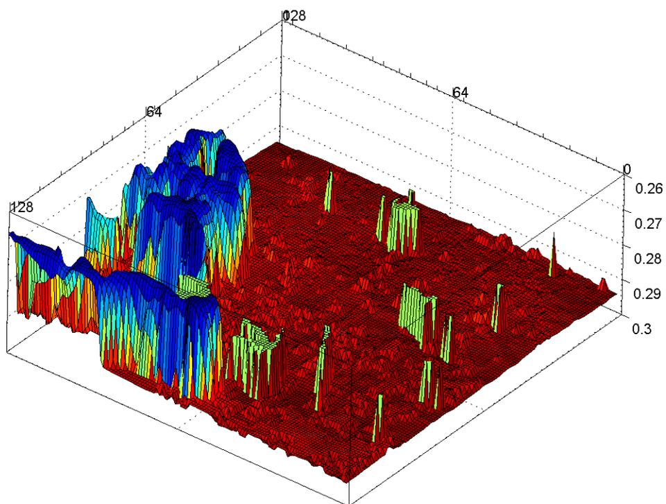
Figure 10. Same blackbody calibration error data as the right hand panel of Fig. 9, but shown here as a three-dimensional surface plot. The internal blackbody calibration error at  $900\text{ cm}^{-1}$  varies across the scene due to the presence of clouds in the simulation. The “peaks” in the surface represent a decrease in the error in the absolute calibration of the GIFTS radiances for the colder cloudy scenes. All units are in Kelvin.
