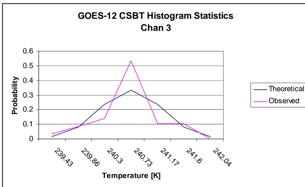
**Figure 3B.** Distribution of Observed (red) clear FOVs (N=50) after a “Gaussian fit” correction has been applied. Average Temperature for Band 3 (6.5 $\mu$ m) is 240.73K.
