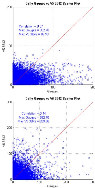
Figure 14. Scatter plots of TG vs V5 and V6 3B42
