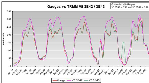
Figure 5a. Time series of average rain rate over Thailand for Thailand gauge, V5 3B42 and 3B43.
