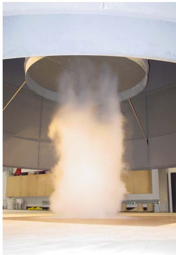
Figure 1: Tornado simulator with vortex highlighted through the use of dry ice.
