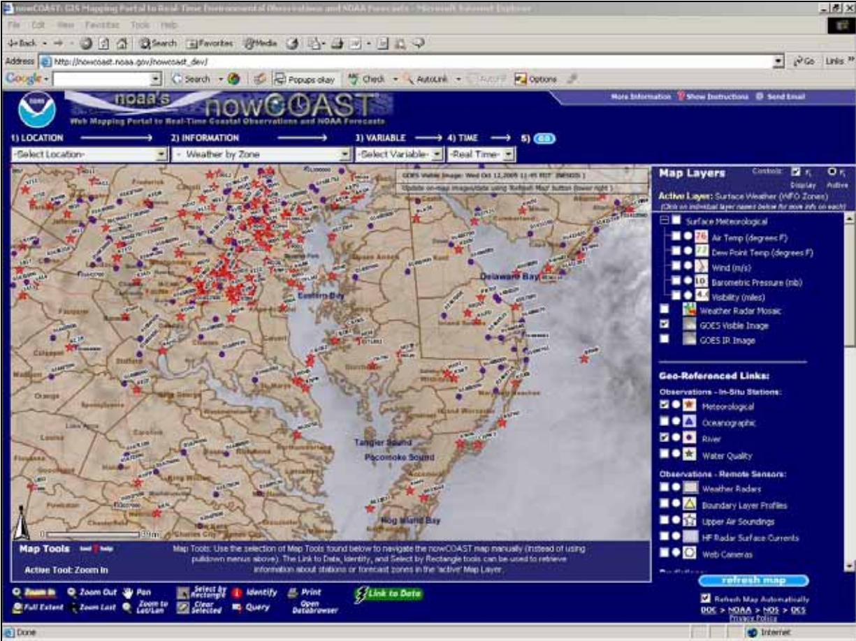
Figure 4. An example of a nowCOAST Map Comparing Distribution of Weather and River Observation Stations overlaid on top of NWS Surface Weather Forecast Regions along with Visible Satellite and Composite Radar Images in the Lower Potomac River Watershed.
