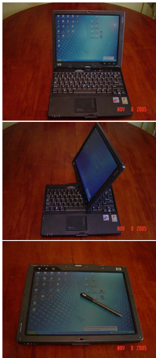
Figure 1. Tablet PC with full keyboard display and modified to a writing tablet.
