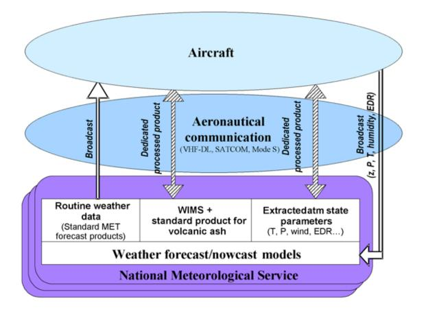
What the diagram shows is that three data flows are envisaged – so-called routine weather data, WIMS products (plus volcanic ash) and atmospheric state parameters.
