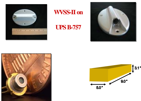
Figure 1. The three main components of the WVSS-II: the air sampler (top), the diode laser assembly (lower left), and combined measurement cell and electronics box (lower right). The two connecting hoses from the air sampler to the electronic box are not shown.
