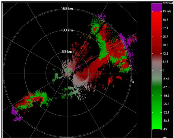
**Fig. 3.** Doppler velocity field corresponding to the Batch mode. Displays encode positive velocities (away from the radar) with red; more intense colors correspond to larger Doppler velocities. Purple indicates a non-recoverable overlaid return.
