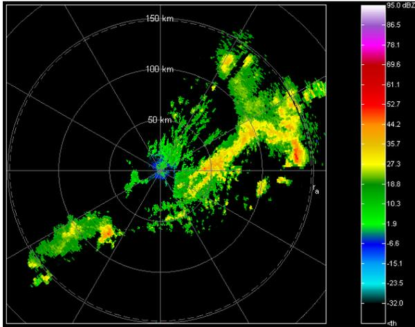
**Fig. 2.** Reflectivity field corresponding to the Batch mode (2.5 deg elevation). Range rings are 50 km apart.
