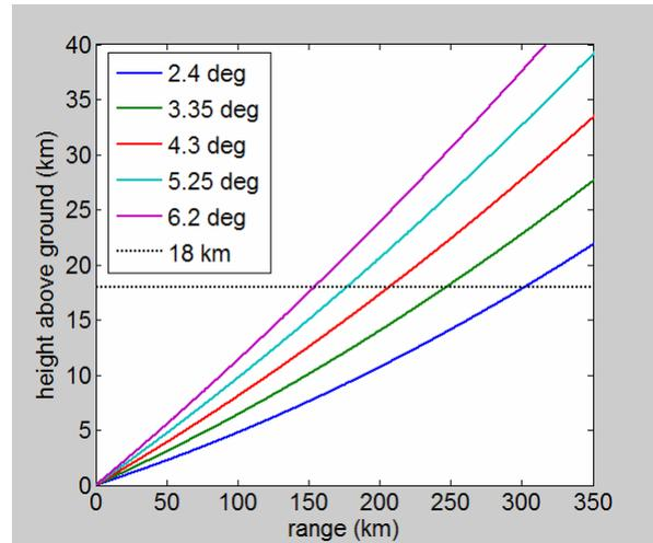
Fig. 1. Required maximum range coverage for different antenna beam elevation angles assuming maximum height of storm tops at 18 km (~59000 ft). Depicted antenna elevation angles are typically processed using the WSR-88D batch mode.
