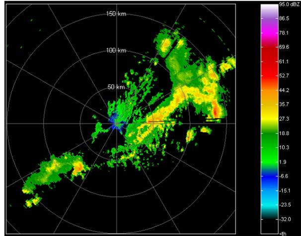
**Fig. 4.** Reflectivity field corresponding to the Staggered PRT algorithm (2.5 deg elevation).
