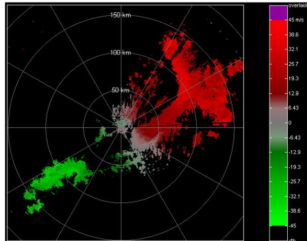
**Fig. 5.** Doppler velocity field corresponding to the Staggered PRT algorithm.
