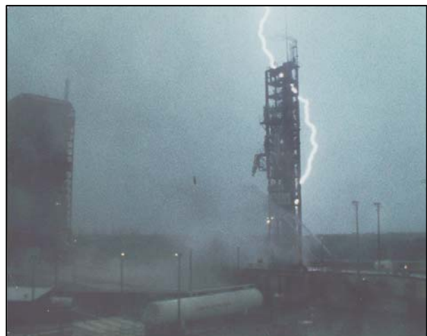
Figure 3. Triggered lightning strike to AC-67 in 1987. The lightning followed the exhaust plume to the ground.
