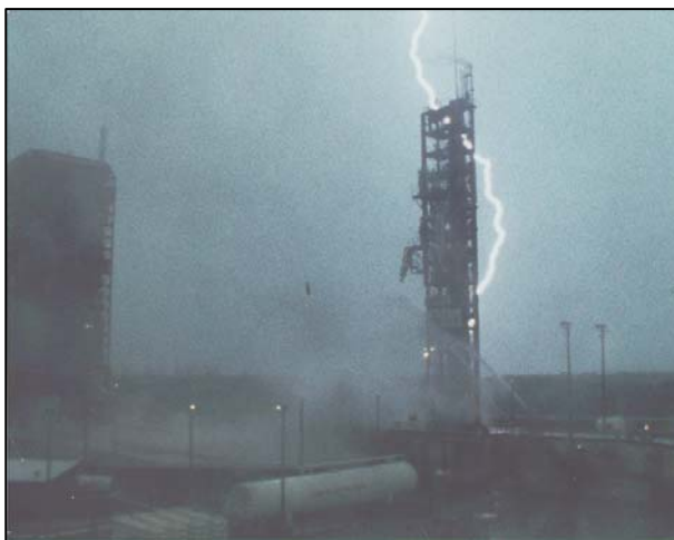
Figure 3. Triggered lightning strike to AC-67 in 1987. The lightning followed the exhaust plume to the ground.
