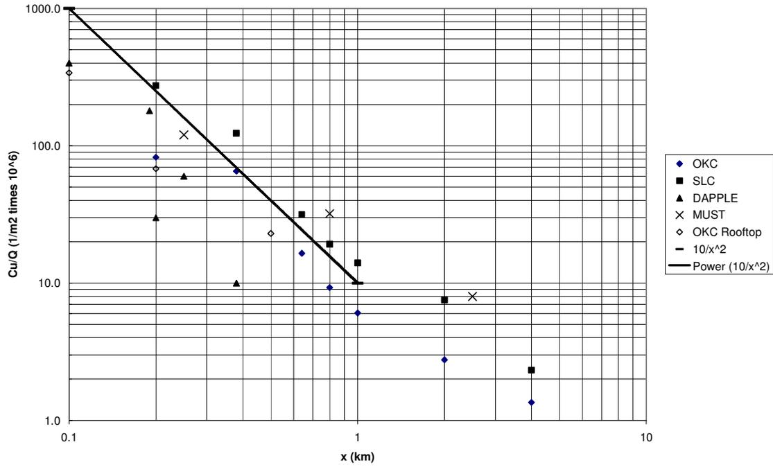
Figure 4. Summary plot of Cu/Q versus x for four field data sets (OKC, SLC, London DAPPLE, and MUST). C is the maximum 30-minute averaged concentration observed along a cross-wind arc of monitors at a given downwind distance, x. The line given by  $Cu/Q = 10/x^2$  is drawn, which Neophytou and Britter (2004) and others have suggested as valid for  $x/H < 50$ , or for  $x < 1000$  m when mean building height, H, is 20 m.
