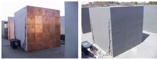
Figure 3 Direct measurements of conductive heat flux (G) using very thin heat plates
