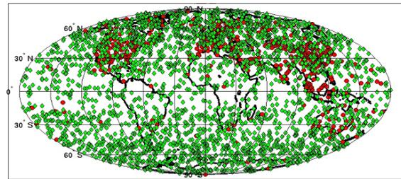
**Figure 3.** The FORMOSAT-3/COSMIC constellation monitors as many as 2,500 profiles of the atmosphere each day. In comparison, terrestrial sounding stations provide only 900 profiles of measurements (red dots).
