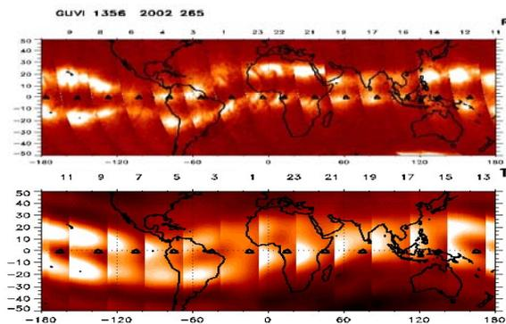
Figure 7. Observing nighttime (23LT) electron density structure using the photometer and ground-based GPS receivers. (Top: 135.6 nm emission collected on TIMED satellite; Bottom: GPS TEC)
