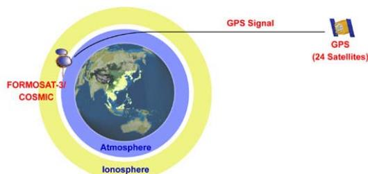
**Figure 2.** The FORMOSAT-3/COSMIC GPS radio occultation technique.
