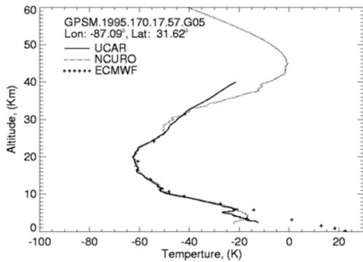
Figure 6. The comparison of dry temperature profiles which were retrieved by UCAR(solid) and NCURO and ECMWF(+) model. The temperature difference above 25 km is due to the different background climatological models be used.
