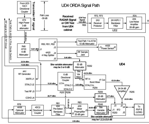
Figure 1: ORDA Receiver Signal Path
