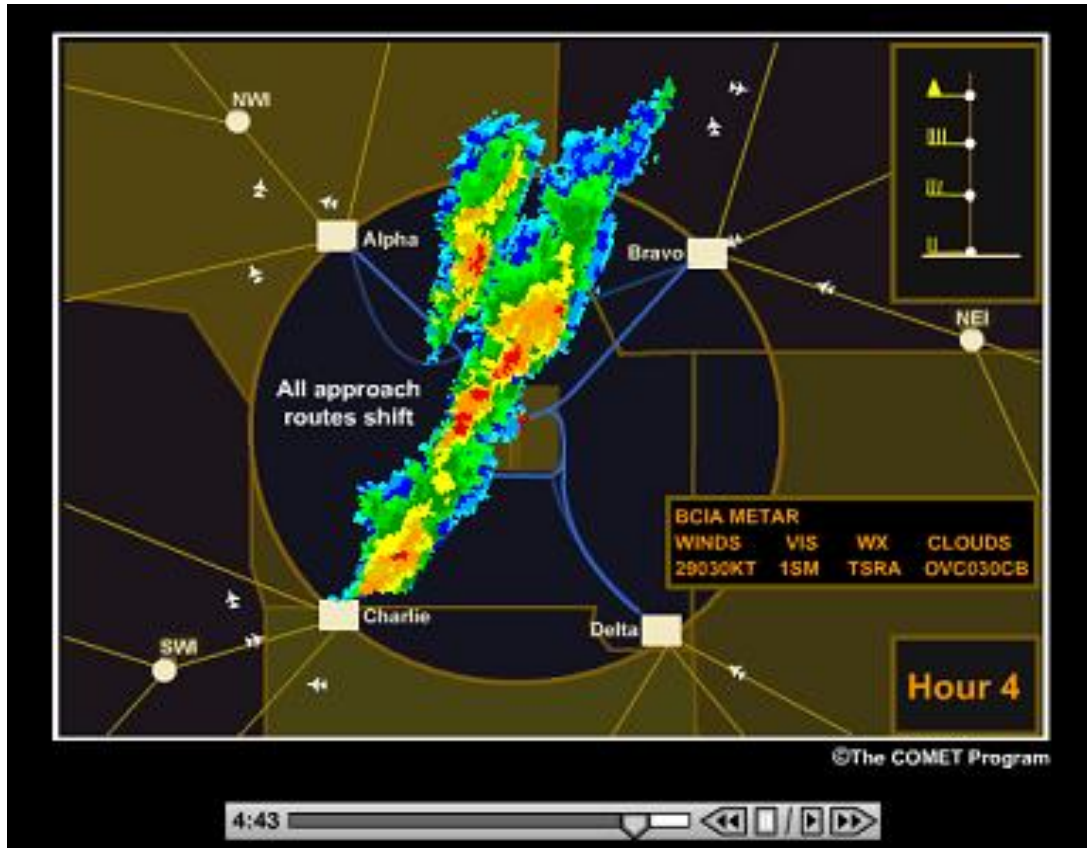
Figure 8 Major airport scenario at a later time, showing impact to traffic from squall line. Aircraft at Alpha, Bravo, Charlie, and Delta arrival gates are holding due to the weather.
