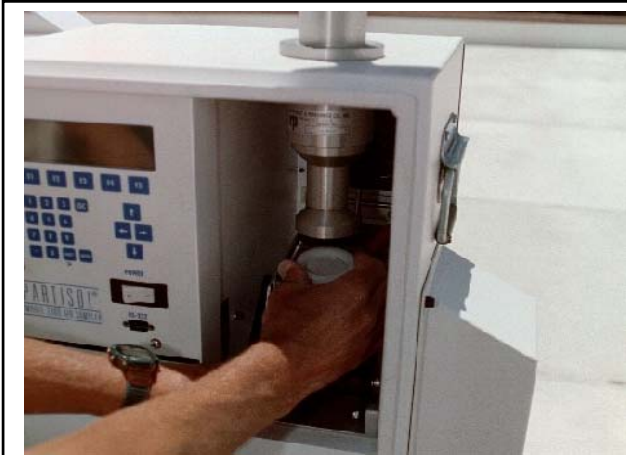
Figure 4. An aerosol sampler used for determination of particulate optical extinction characteristics.
