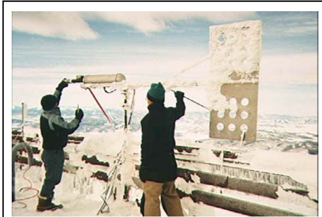
Figure 2. A University of Nevada, Reno student (left) and UNR/DRI faculty member (Dr. Randy Borys, right) conducting a calibration procedure for a vane-mounted cloud optical probe at DRI Storm Peak Laboratory in northern Colorado.
