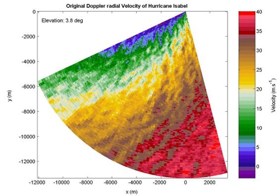
Figure 1: Original Doppler radial velocity data from Hurricane Isabel collected by SMART radar 2 (SR2).
