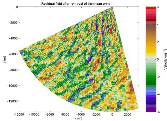
Figure 3: Radar velocity residuals after removing the mean wind filed using the VAD technique for Hurricane Isabel.
