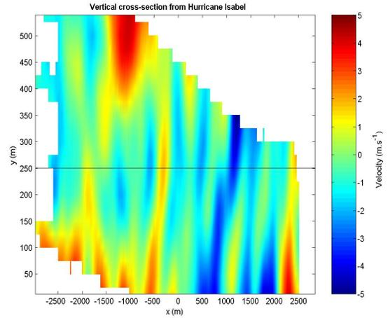
Figure 9: Vertical cross-section of radial velocity residuals taken from the cartesian gridded data. The solid black line indicates the position of the data shown in Figure 11.
