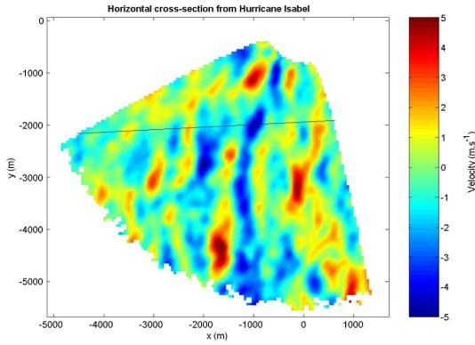
Figure 7: Horizontal cross-section taken at 300 m AGL after cartesian gridding of the volume scan data with a Cressman scheme. A radius of influence of 150 m was used. The solid black line indicates the position of the vertical cross-section shown in figure 9.
