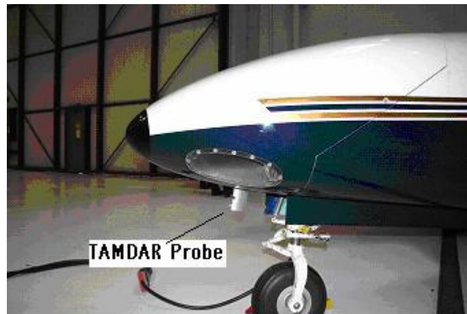
Figure 8 TAMDAR Probe on Piper Seminole Nose
