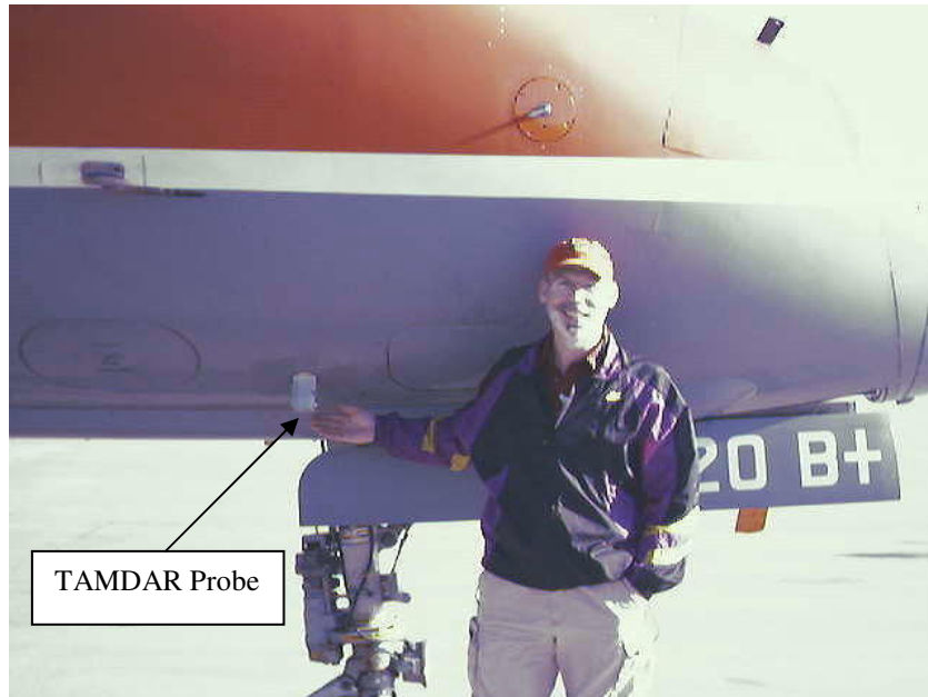
Figure 13 TAMDAR Probe on SAAB 340 Fuselage
