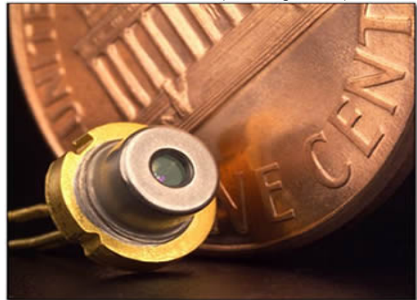
Fig. 1 WVSS-II laser diode shown next to a penny, for size comparison purposes.
