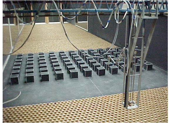
Figure 2. USEPA wind-tunnel interior showing the 7x11 cubical building array. View looking into the wind.
