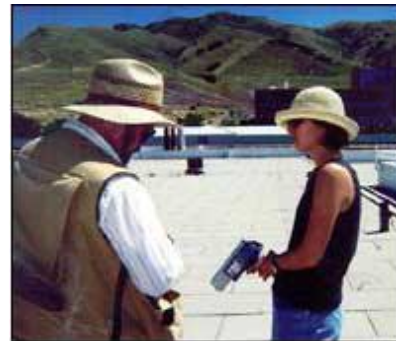
Figure 6. Measuring the albedo of a cool roof in Salt Lake City, UT. (US EPA HIRI web site).
