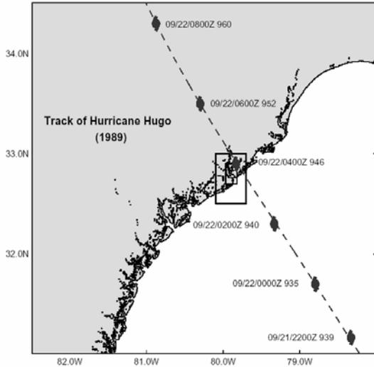
**Figure 2** The setup of nesting domain and the best track of hurricane Hugo.
