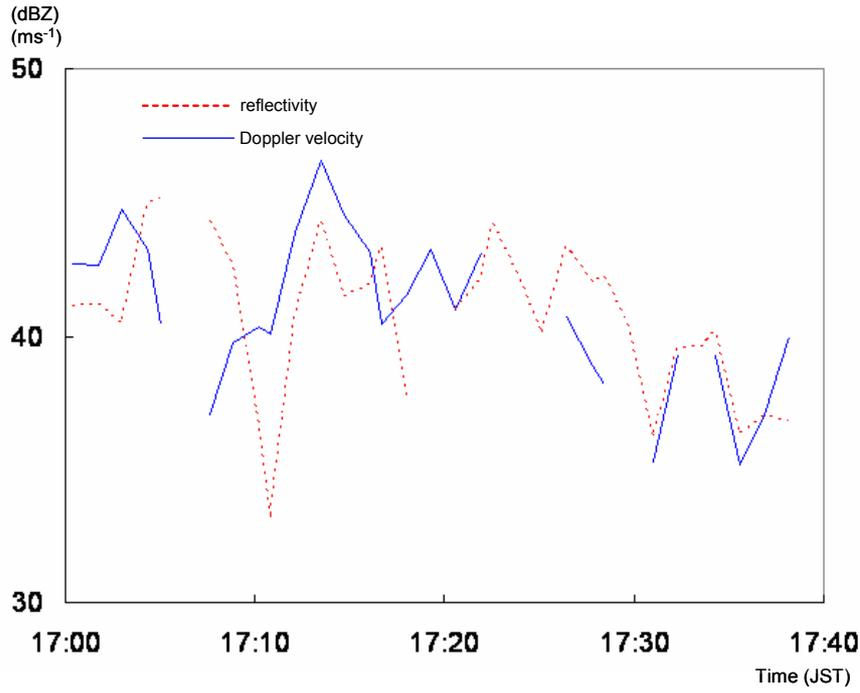
FIG. 6. The 75-sec time plots of radar reflectivity and Doppler velocity at 700m altitude (the lowest elevation is 0.8°) over the Nago Observatory. Note that the Doppler velocity data are absolute values.
