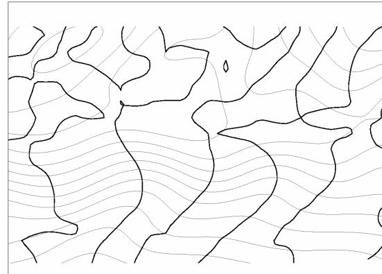
**Figure 4** - Contours where the advection of streamfunction curvature vorticity by the non-divergent wind is equal to zero (equation (6), thick black lines) on top of source  $\psi$  field (grey contours).
