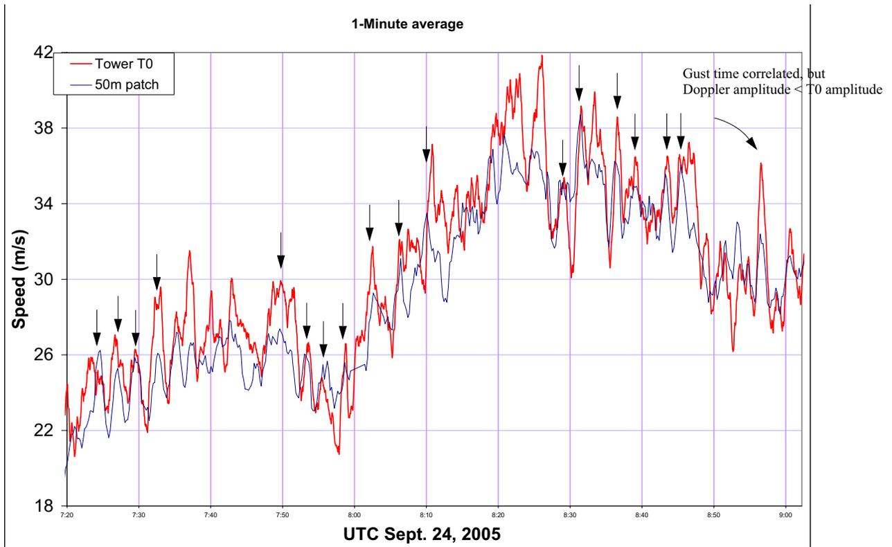
Comparison of Doppler and FMCP T0 winds over shorter time period to illustrate qualitative alignment of 1-min period gusts. Amplitude of 1-min variability is higher at T0, probably due to inadequate spatial averaging method for Doppler patch. (soon to be corrected) Same 0.7 normalization and cosign corrections applied.
