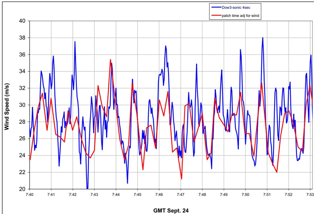
Comparison of DOW3 sonic anemometer winds, 4 s average, with upstream Doppler winds averaged over a 50 m radius circle at 200 m range. 4 s anemometer averaging chosen to correspond to 100 m trajectory @ 25 m/s. At 1.2°, 200 m range is about 7 m above DOW wheel level. An 8 s lag is applied to the Doppler data to allow for parcel propagation to the anemometer (200 m @ 25 m/s).
