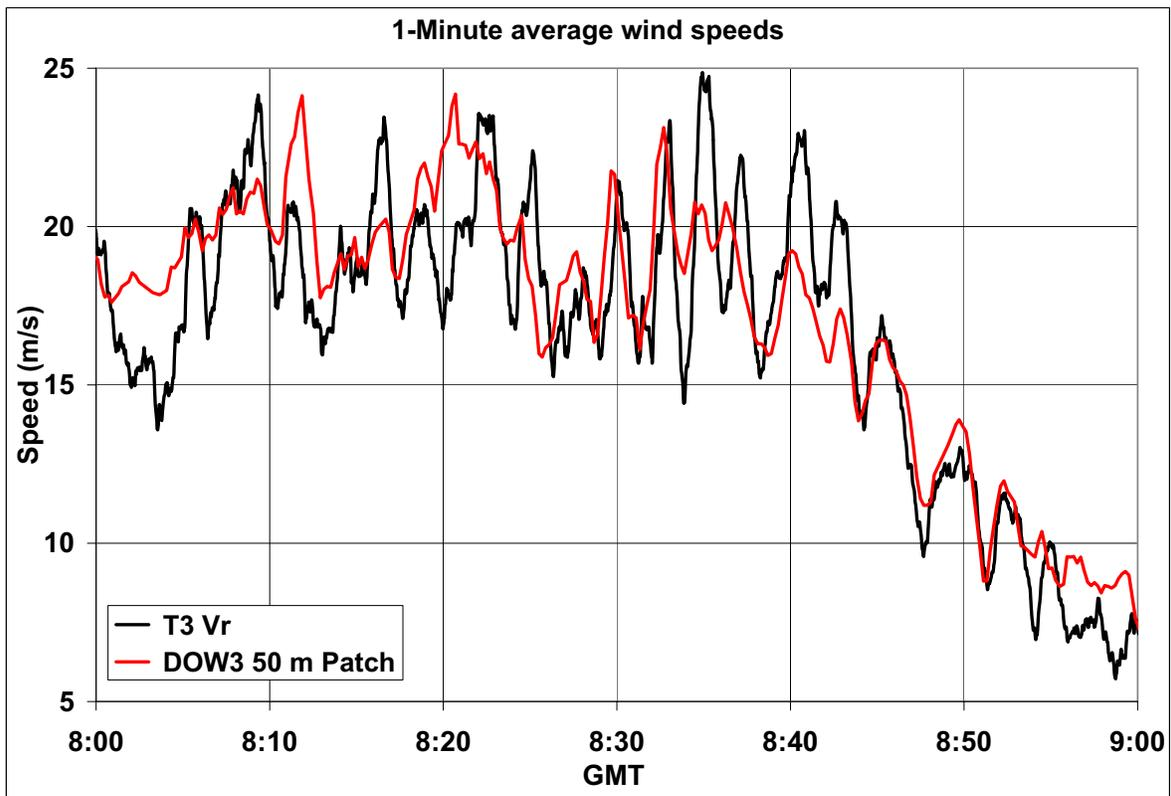
Similar DOW Doppler and FCMP T3 comparison. 0.43 normalization for apparently more sheltered location applied as well as cosine correction. 1-min gusts seem to be well correlated.
