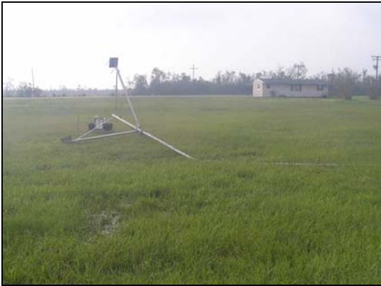
Figure 10. Photograph of the damaged PMT at Orange County Municipal Airport, Orange, TX.
